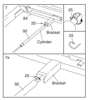
8. Raise the Gas Spring (92) to a vertical position. Remove the Spring Pin (25) from the raised end of the Gas Spring as described in step 7. If necessary, rotate the Gas Spring to align the end of the Gas Spring with the ball on the bracket on the Frame (58).
